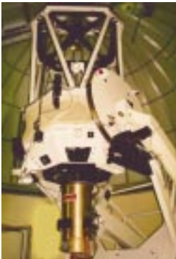
Top: The 2MASS 1.3-meter telescope in the southern hemisphere sits high in the Andes at the Cerro Tololo Interamerican Observatory. Inside the dome (above) the camera, with its massive arrays of detectors and filters for three wavelengths, is attached to the back of the telescope.
